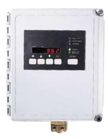
The AquaMatic 962 Stager Controls combine an AquaMatic Stager with an Autotrol® 962 Series Electronic Control, mounted and prewired in a NEMArated enclosure. The AquaMatic Stager is a rotary pilot valve with multiple ports for directing fluid flows to operate various diaphragm valves installed in a water treatment system. AquaMatic Stager internal parts are constructed of durable, non-corroding, selflubricating materials for long, maintenance-free life.
