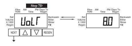
Step 7D - Display shows the latest measured voltage of the battery pack. Pressing and holding the ▲ and ▼ buttons simultaneously for approximately 5 seconds will initiate a test of voltage. (Normally this test is automatically conducted at 12:00 am daily.)
