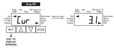
Step 9D - Display shows the present measured charge current of the solar panel, measured in mA. An active Set Arrow indicates that the control is currently determining whether to activate the charging circuit. Active Set and Fill Arrows indicate that the charging circuit is currently activated. Pushing ▲ once temporarily turns on the charging circuit, and activates the SET and FILL arrows. Pushing ▼ temporarily turns off the charging
