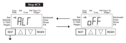
Step 6CS – Allows selection of one of the following using the ▲ or ▼ buttons:
