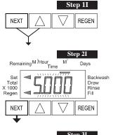
**Step 1I** - To enter Installer Display press NEXT and ▲ simultaneously for 5 seconds and release.
