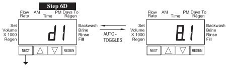
Step 6D - Display shows the daily voltage level of the battery pack. The first display is the day and the second display is the voltage. The voltage is recorded at midnight. The number of days ranges from 1 to 127. Press NEXT to go to Step7D. Press REGEN to return to previous step.
