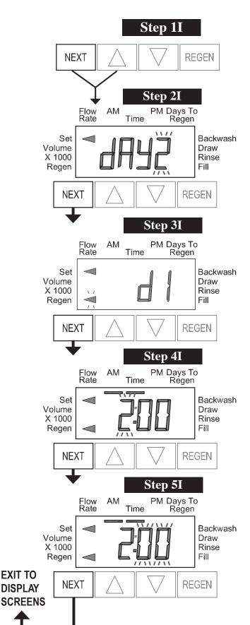
**Step 1I -** To enter Installer Display press the NEXT and **▲** buttons simultaneously for 5 seconds and release.
