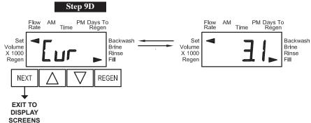
Step 9D - Display shows the present measured charge current of the solar panel, measured in mA. An active Set Arrow indicates that the control is currently determining whether to activate the charging circuit. Active Set and Fill Arrows indicate that the charging circuit is currently activated. Pushing ▲ once temporarily turns on the charging circuit, and activates the SET and FILL arrows. Pushing ▼ temporarily turns off the charging circuit.
