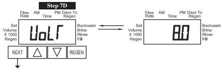
Step 7D - Display shows the latest measured voltage of the battery pack. Pressing and holding the ▲ and ▼ buttons simultaneously for approximately 5 seconds will initiate a test of voltage. (Normally this test is automatically conducted at 12:00 am daily.)
