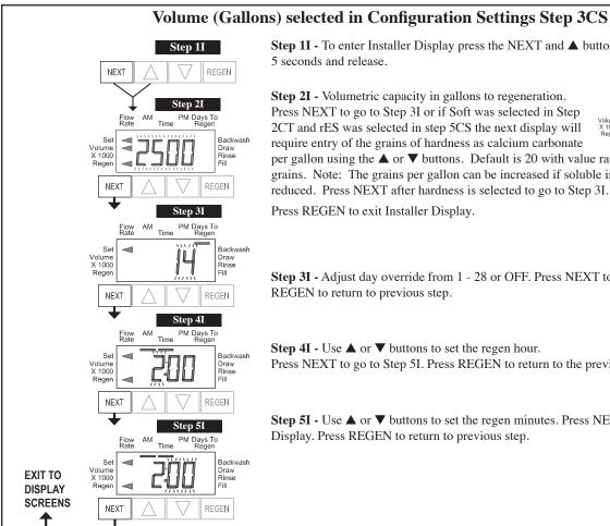
Step 1I - To enter Installer Display press the NEXT and ▲ buttons simultaneously for 5 seconds and release.
