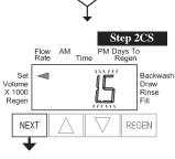
**Step 2CS** – Choose 1.0 for 1", 1.25 for 1.25", 1.5 for 1.5", 2.0L for 2L, 2.0 for 2" valve. Press NEXT to go to Step 3CS. Press REGEN to exit Configuration Settings.
