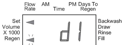
**Step 3I** - Scroll through days 1 to 7 using NEXT. Use ▲ or ▼ to turn regen on or off for each individual day (regen indicator on means regeneration will happen). After completing the 7th day, press NEXT to go to Step 4I. Press REGEN to go to previous display.
