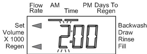
**Step 4I** - Use ▲ or ▼ to set the regen hour. Press NEXT to go to Step 5I. Press REGEN to go to previous display.
