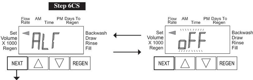
Only use Clack No Hard Water Bypass Valves or Clack Motorized Alternating Valves (MAV) with these selections. Clack No Hard Water Bypass Valves (1" or 1.25" V3070FF or V3070FM) are not designed to be used with the alternator or separate source functions. The V3063 and V3063BSPT motorized alternating valves are not designed to be used as a no hard water bypass or separate source inlet if the pressure differential is more than 60 psi.
