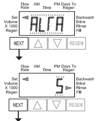
For Clack Corporation alternator systems using the WS2 valve, when NEXT is pressed after selecting ALTA or ALTB, a display will allow the user to set the amount of pre-service rinse time for the stand by tank just prior to returning to service.
