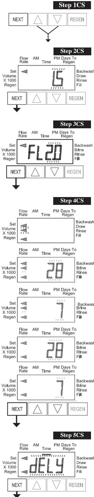
**Step 1CS** – Press ▲ and ▼ simultaneously for 5 seconds and release. If screen in Step 2CS does not appear, the lock on the valve is activated. To unlock press ▼, NEXT, REGEN, ▲ in sequence, then press ▲ and ▼ simultaneously for 5 seconds and release.
