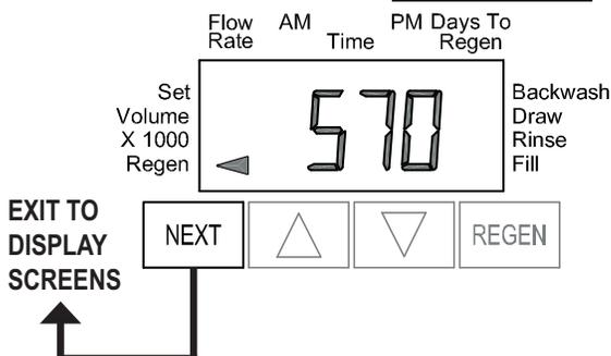
**Step 1D** - Press ▲ and ▼ simultaneously for 5 seconds and release. Then press ▲ and ▼ simultaneously for 3 seconds and release. If screen in Step 2D does not appear the lock on the valve is activated. To unlock press ▼, NEXT, REGEN, ▲ in sequence, then press ▲ and ▼ simultaneously for 5 seconds and release. Then press ▲ and ▼ simultaneously for 3 seconds and release.
