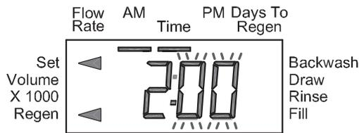
**Step 5I** - Use the ▲ or ▼ to set the regen minutes. Press NEXT to exit Installer Display. Press REGEN to return to previous display.
