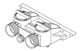
To return to the conditioned water or service position, rotate the handles counterclockwise so they are parallel to the flow path of the inlet and outlet water stream, as shown below.
