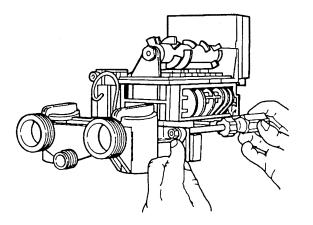
3. Connect bypass valve to tank adapter using (4) nuts and bolts as shown.
