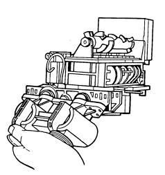
2. Slip bypass valve over O-rings into position.
