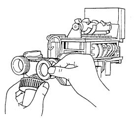
4. Insert tailpieces through union nuts. Attach tailpieces into inlet and outlet piping. Place rubber washer in nut and thread to bypass valve body. It is not necessary to lubricate or use sealant on rubber washer or union nuts.
