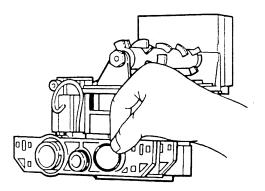
1. Apply O-rings (3 required) to tank adapter. Lubricate O-rings with silicone lubricant.
