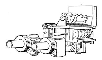
5. After all plumbing connections have been made, the rotor handles should be turned to the service position as shown (handles aligned with flow arrows).
