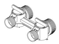
To return to the conditioned water or service position, rotate the handles counterclockwise so they are parallel to the flow path of the inlet and outlet water stream, as shown below.
